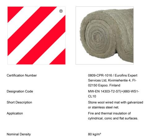
PAROC stone wool products are capable of withstanding high temperatures. The binder starts to evaporate when its temperature exceeds approximately 200°C. The insulating properties remain unchanged, but the compressive stress weakens. The softening temperature of stone wool products is over 1000°C.
